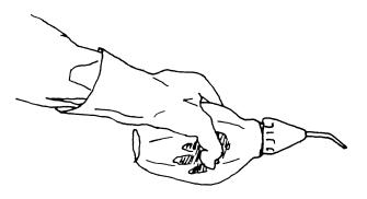
**Plunger dusters** hold more dust than the first two hand-held dusters discussed. Plunger-type dusters have been used for garden dusting for a century, but the plunger duster used in structural pest management is smaller, made of high-impact plastic, and has several styles of nozzles.
