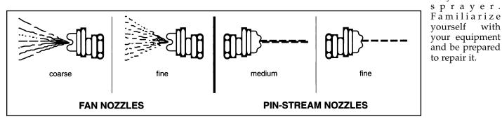
Figure 2-3. The spray patterns produced by the fan and pin-stream orifices on a four-way nozzle tip.
