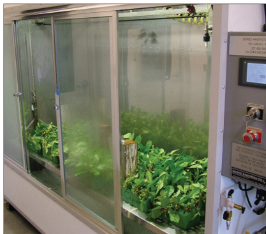
Fungicide-treated montmorency cherry shoots are exposed to rainfall in the rain simulator at TNRC.
