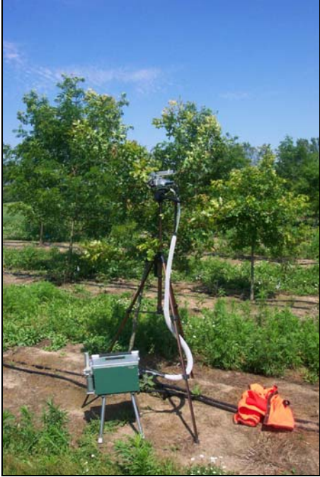
Figure 3. Gas exchange measurements with a Li-6400 portable photosynthesis system.
